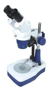
Objective : Grouped From Any Two Objectives of 1X, 2X, 3X and 4X, Working Distance : 12
