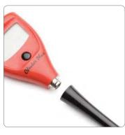
The HI1271 pH electrode can be easily replaced. Just unscrew the electrode from the meter body and screw on a new one.
