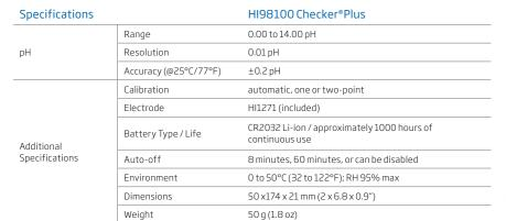
Ordering Information **HI98100** (Checker Plus) is supplied with HI1271 pH electrode, pH 4.01 buffer solution sachet (2), pH 7.01 buffer solution sachet (2), electrode cleaning solution sachet (2), battery, quality certificate, and instruction manual in a carrying case.
